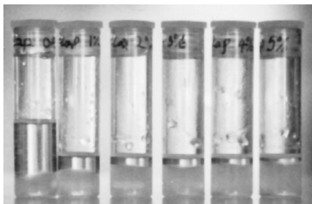
Figure 3. Phase separation after 40 h. From left to right: 0.5, 1, 2, 3, 4 and 5 wt% of DODAB stabilized Laponite in K15.
